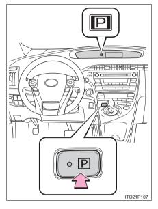
Push the "P" position switch with the brake pedal pressed down.
