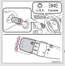
The side marker, parking, tail, license plate and instrument panel lights turn on.
