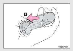
Wash/wipe operationWipers operate automatically.
