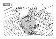
If necessary, add power control unit coolant up to the full line.
