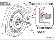
Install the spare tire and loosely tighten each nut by hand to approximately the same amount.
