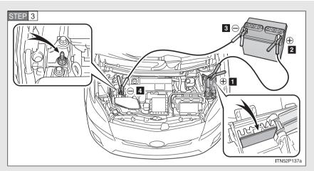
Connecting the jumper cables.
