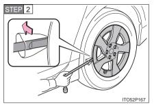
Vehicles with a 15 inch wheel, remove the wheel ornament using the wrench.
