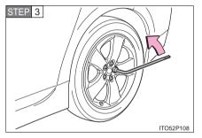
Slightly loosen the wheel nuts (one turn).
