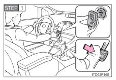
Apply the brakes and touch the Toyota emblem side of the electronic key to the "POWER" switch.
