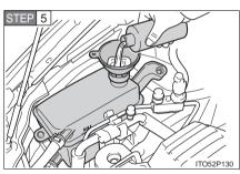
If necessary, add engine coolant up to the "FULL" line.
