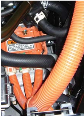
High-Voltage Cable Connection to Motor
