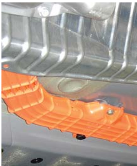
Electrical shield bolted to undercarriage
