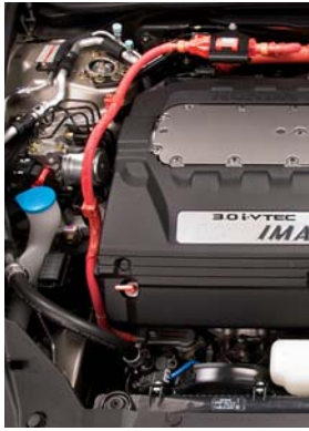
High-Voltage Cable to Accord AC Compressor
