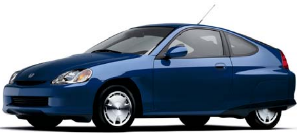
The Insight is a 2-passenger car with a distinctive aerodynamic shape and rear fender skirts.
