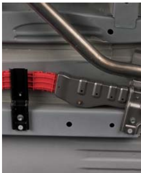
Thermal shield near hot exhaust
