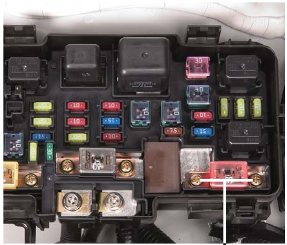
Main Fuse Screws
