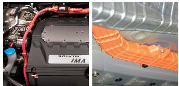
Orange cables under the hood, or orange shielding bolted to the undercarriage of a Honda, tell you the vehicle is a hybrid.
