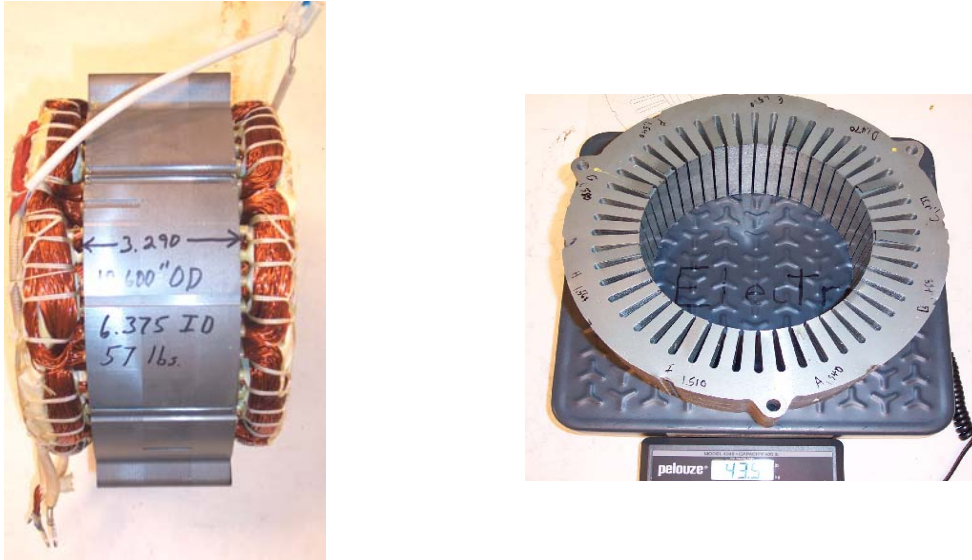
Fig. 7. Prius 2004 wound stator and its stator core.
